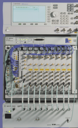
Figure B Agilent Technologies' 40/100-Gbps BER tester lets you test physical layers for bit errors.
